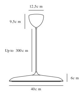
Voltage (V): 220-240 Volt IP degree: IP20 Class (Class 1, Class 2, Class 3): Class 2 (Double isolated) Socket type: LED Module
