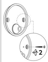
Fasten mounting bracket to surface using supplied M4x30 screws and ensure washers are in screw holes
