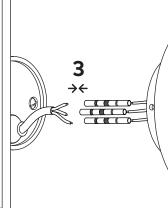
Match polarity and connect L-E-N using provided Heatsink Solder Joiners (Refer to wiring)
