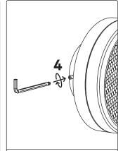
Attach luminaire to mounting bracket and tighten screws using provided allen key to complete installation.
